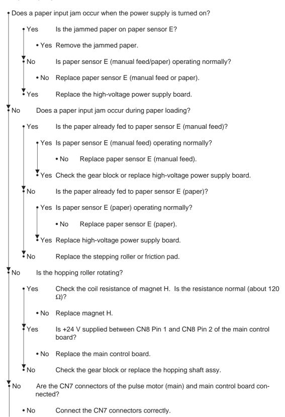
Yes Measure the resistance of the pulse motor (main). Is the resistance normal (about 12.6 Ω)?
